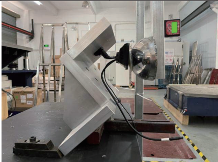
Fig.12 Test setup- 6# (Frontal Impact)
