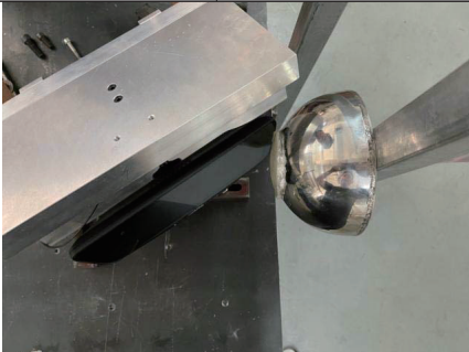
Fig.15 Test setup- 8# (45 ° angle Impact)
